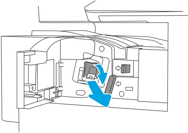
3. Lift two tabs on the staple cartridge, and then lift up to remove the empty staple cartridge from the staple cartridge carriage assembly.
