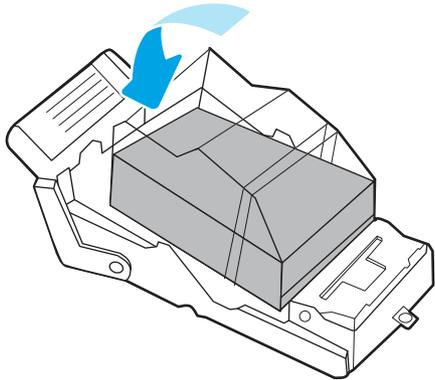
6. Hold the knob to immobilize the staple cartridge assembly, insert the new staple cartridge into the assembly, and then press the colored handle inward until it snaps into place.
