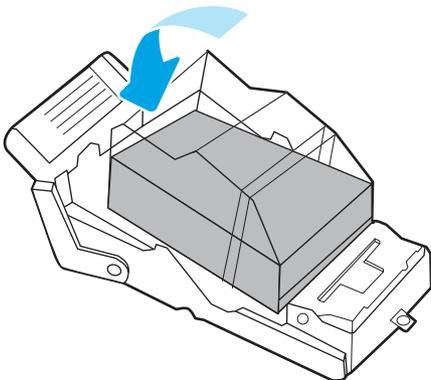
5. Reinstall the staple cartridge carriage into the stapler by pressing the colored handle inward until it snaps into place.
