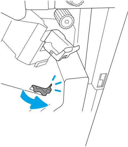
3. Hold the knob to immobilize the staple cartridge assembly, grasp the colored tab on the staple cartridge carriage, and then pull the staple cartridge carriage straight out.
