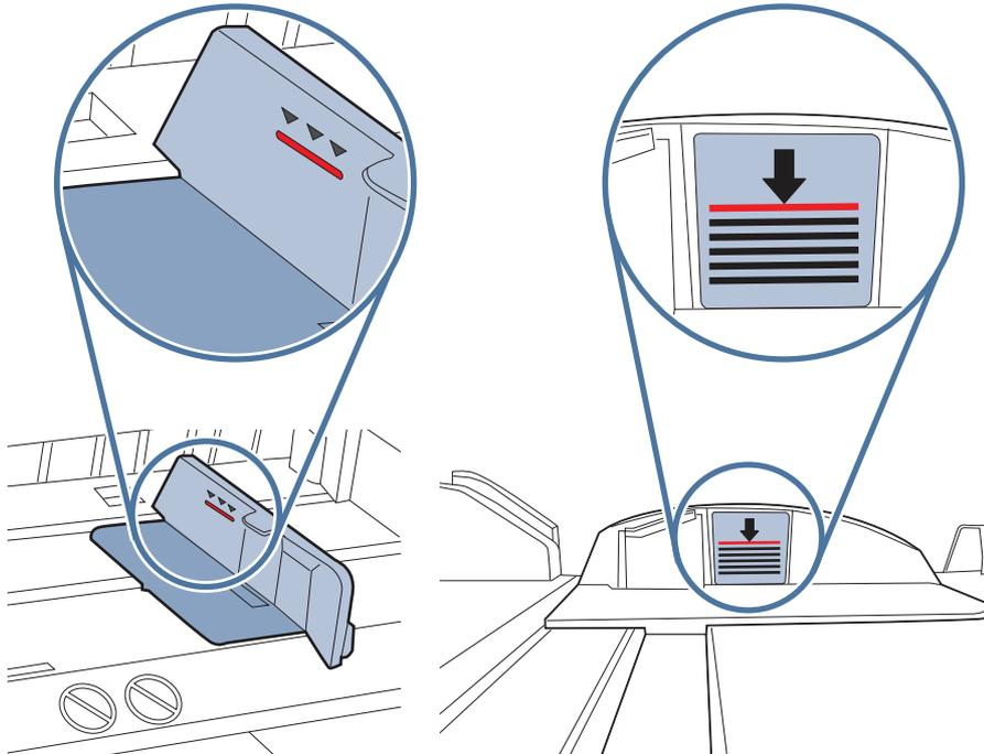
**Figure 9-7** Tab for the paper stack
