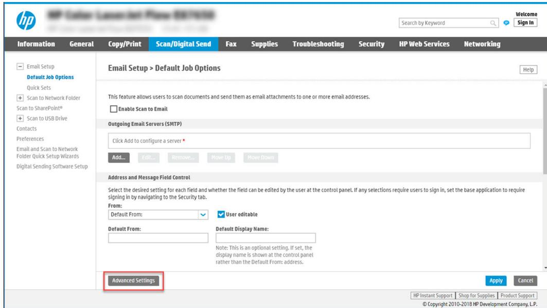
2. On the **Default Job Options** page, select the **Enable Scan to Email** check box. If this check box is not selected, the feature is unavailable at the printer control panel.
