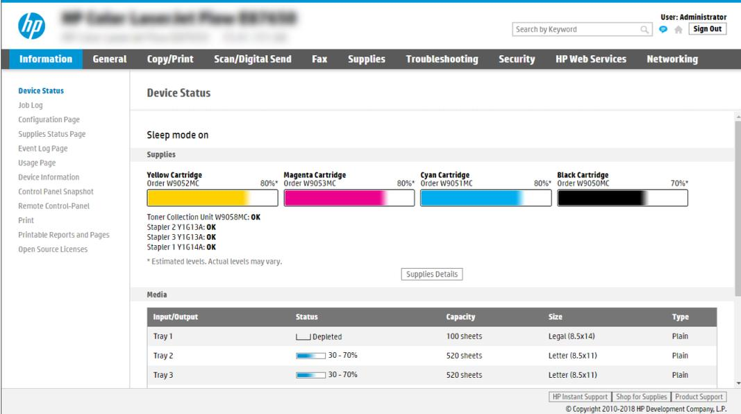
The screenshot displays the HP Embedded Web Server (EWS) interface. The top navigation bar includes tabs for Information, General, Copy/Print, Scan/Digital Send, Fax, Supplies, Troubleshooting, Security, HP Web Services, and Networking. The main content area is divided into sections: Device Status, Supplies, and Media.
