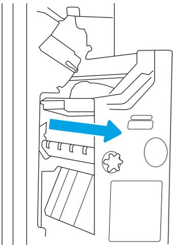
3. Pull the colored tabs away from the assembly, and then pull them up to remove the two staple cartridges.
