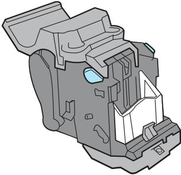
7. Reinstall the two staple cartridge carriers into the booklet maker by pressing the colored handles until they snap into place.
