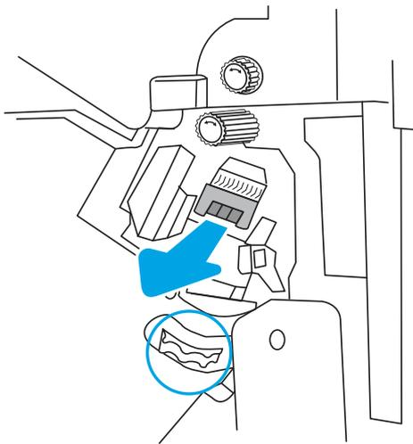
4. Lift two tabs on the staple cartridge, and then lift up to remove the empty staple cartridge from the staple cartridge carriage assembly.
