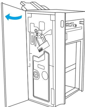
2. Rotate the knob counterclockwise to move the staple cartridge assembly all the way to the front.
